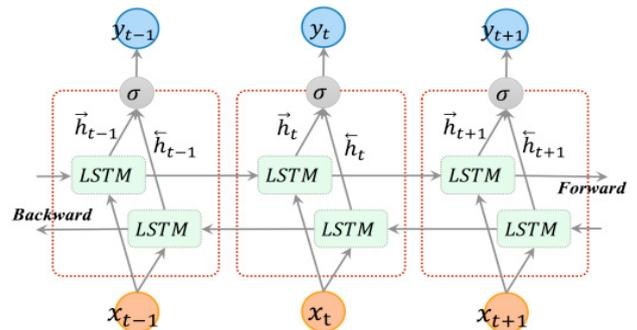
Fig. 3. A Bi-directional LSTM structure(Cui, Ke and Wang, 2018)
