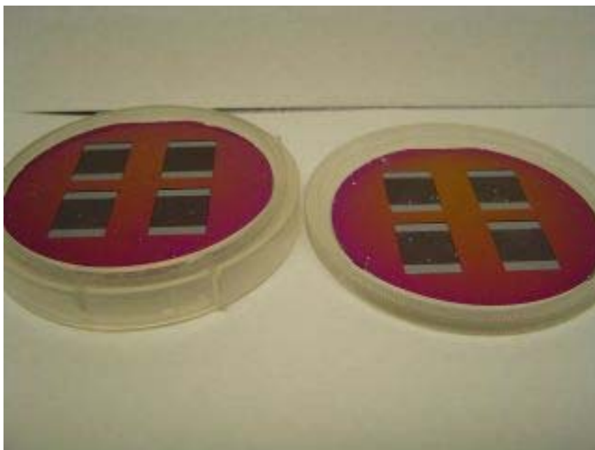
Fig. 5-1 Prototype of Evaporator Lithographically Etched by University of Cincinnati
