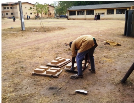
Figure 15 Drying of bricks in the open air. Photograph by Raji, 2015.
