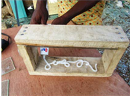
Figure 4 Lacing the mould wall with adhesive. Measuring glass for cutting. Attachment of glass on mould wall. Photograph by Oyewo, 2015.
