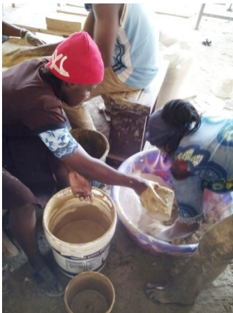
Figure 8 Pouring diluted adobe on powdered kaolin sawdust. Photograph by Oyewo, 2015.
