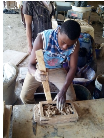
Figure 12 Ramming with wooden shaft. Photograph by Raji, 2015.
