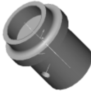
Fig. 4. Grippers for Holding Sand Asphalt Test Specimens
