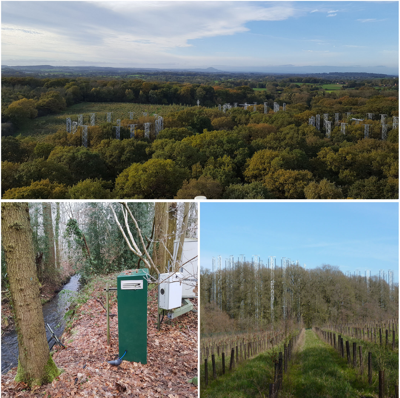
FIGURE 2 Views of the BIFoR FACE catchment. Top: the FACE facility viewed from the top of the 40-m tower, looking southwest. The young plantation containing the fibre-optic cable is visible centre-left of the image. Bottom left: The lower water quality station on Wood Brook. Bottom right: the young plantation, looking northeast, down the rows between which the fibre-optic cable is buried
