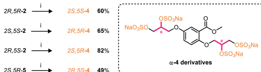
Scheme 4 A chiral pool synthesis of \alpha -4, synthesising each stereochemical combination. Conditions: i) 1) \text{Bu}_3\text{N}\cdot\text{SO}_3 , MeCN, 90 °C, 2) sodium 2-ethylhexanoate, ^t\text{BuOMe}/\text{EtOH} .
