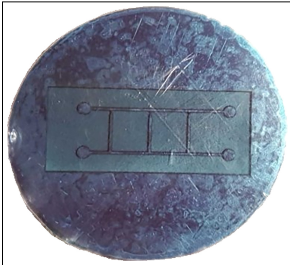
Figure 2. View of the stainless steel negative mould for the manufacture of the PDMS channels.
