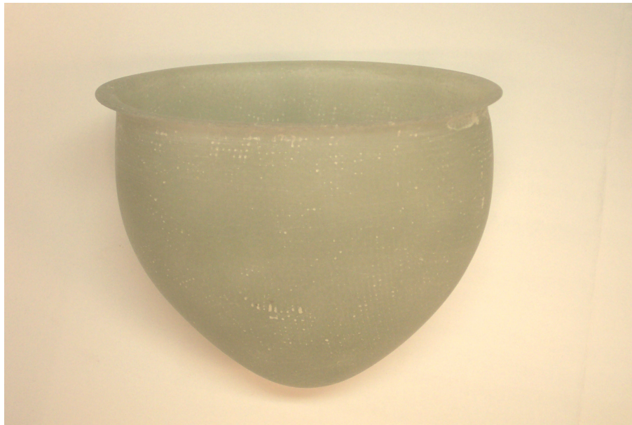
Fig 14. Photograph of the final cup made from the mould
