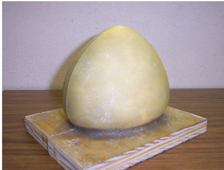
Fig 12. Photograph of the final plug mould
