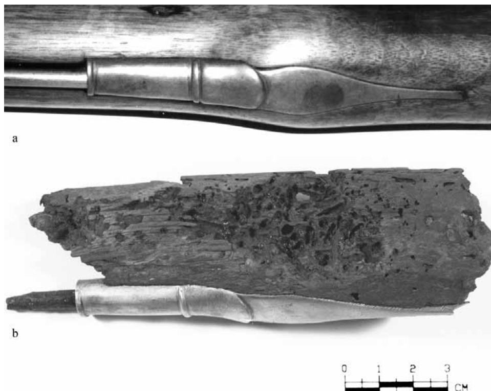
Figure 25. British Barrel Fragment. a) Tailpipe from an Ordnance India Pattern musket (Collection of Bill Caruth, Dallas TX), b) Stock with tailpipe and ramrod, 14992-4. Photography by A. Borgens.
