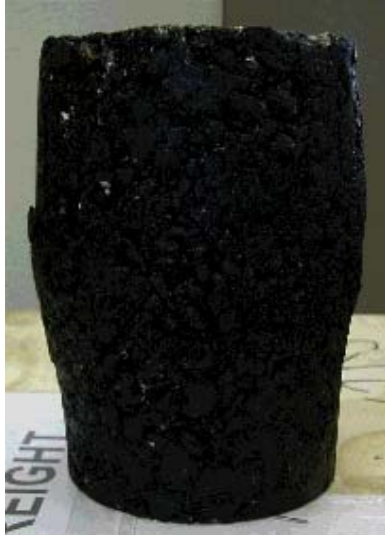
Fig. 5.6. A Deformed AC Limestone Specimen
