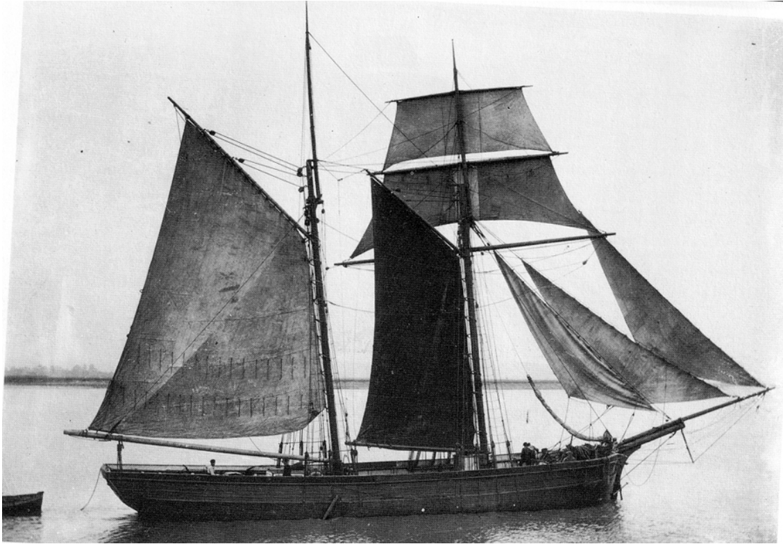
Figure 40. The two-masted fore-and-aft rigged merchant schooner Hope . The vessel is shown with double topsails and no studding sail (From MacGregor 1997, 67).
