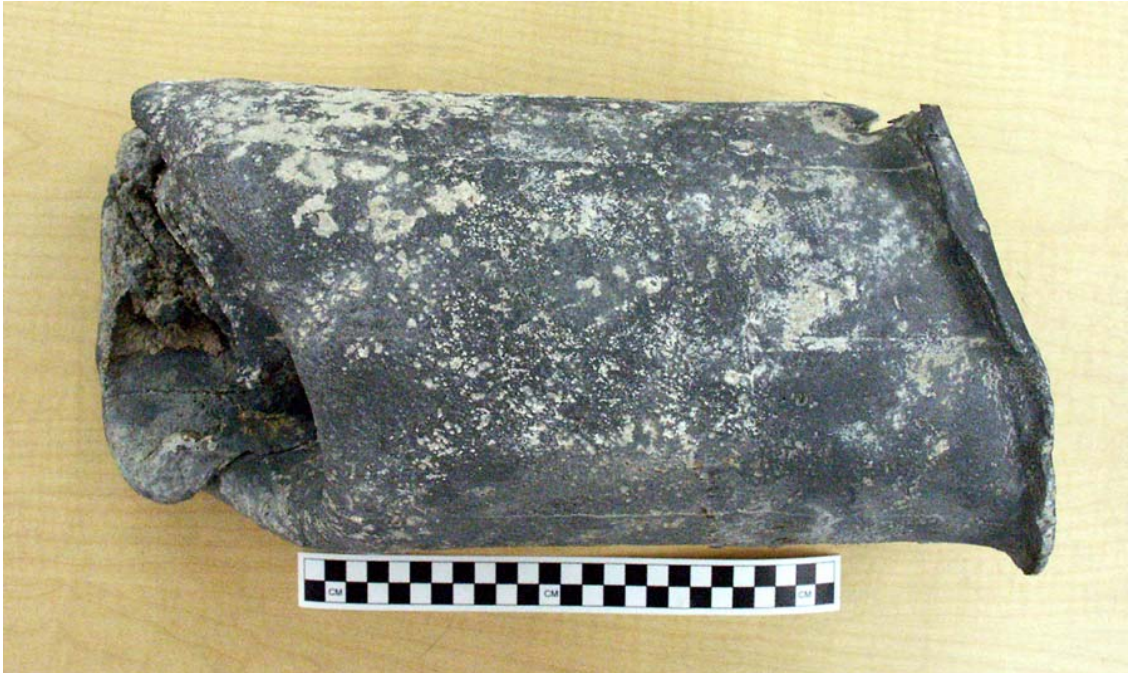
Figure 31. Forward face of lead hawse pipe from the Mica shipwreck. Casting seams are evident on the both the external (right) and internal (left) openings (Photograph by author).
