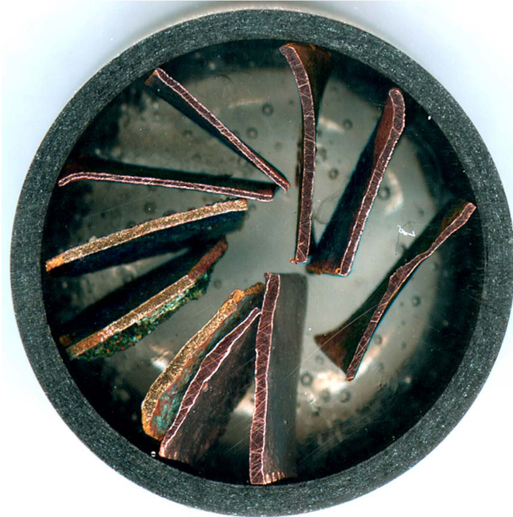
Figure 27. The refracting electron microprobe sample carrier. It contains pieces of metallic sheathing awaiting analysis (Photograph courtesy of Dr. Renald Guillemette).
