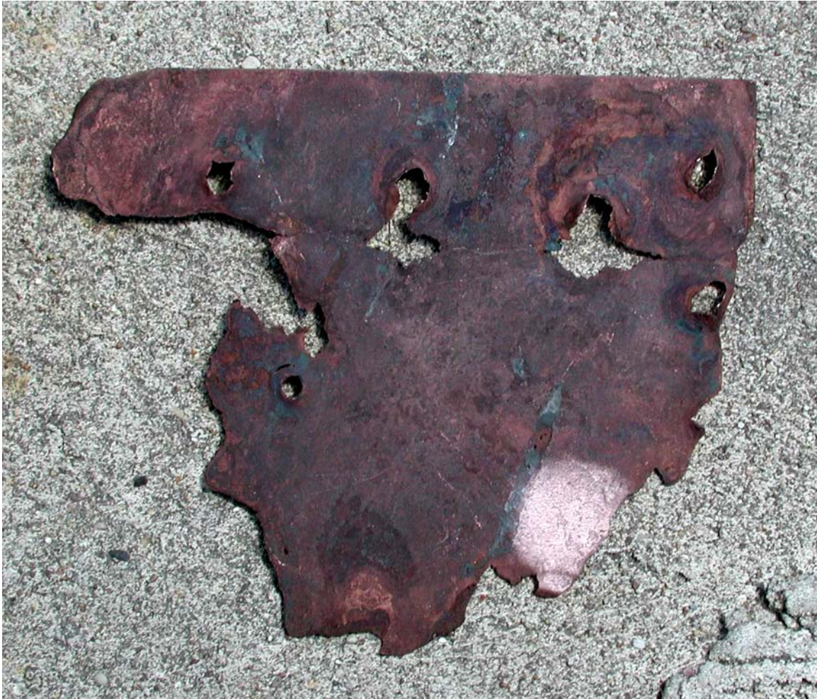
Figure 26. A fragment of the copper sheathing retrieved from the Mica shipwreck. The bright spot in the lower right corner has been mechanically cleaned with a glass bristle brush (Photograph by author).
