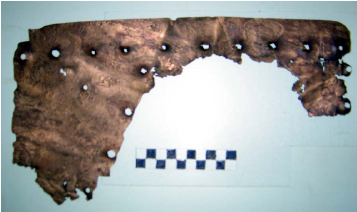
Figure 29. Largest fragment of metallic sheathing recovered from the Mica shipwreck (Photograph by author).
