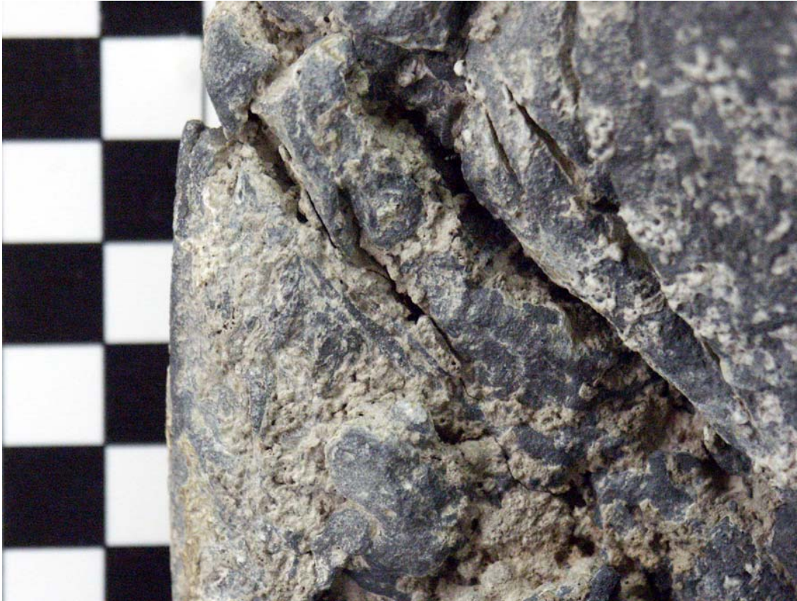
Figure 34. Detail of cut marks near the interior opening of the hawse pipe. Analysis of wear marks and the location of the pipe on the wreck suggested that this was the starboard lead hawse pipe (Photograph by author).
