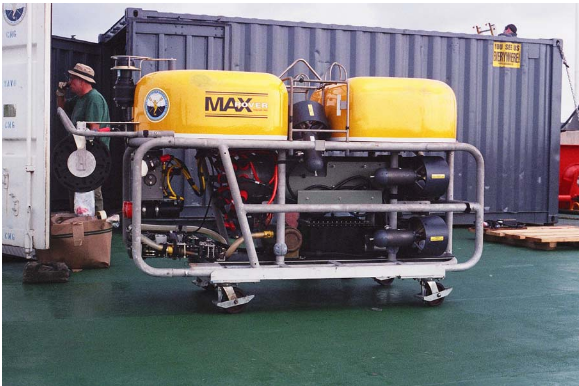
Figure 8. The Naval Oceanographic Office's MaxRover remotely operated vehicle. Here it is seen preparing to explore the Mica shipwreck site (Photograph by author).
