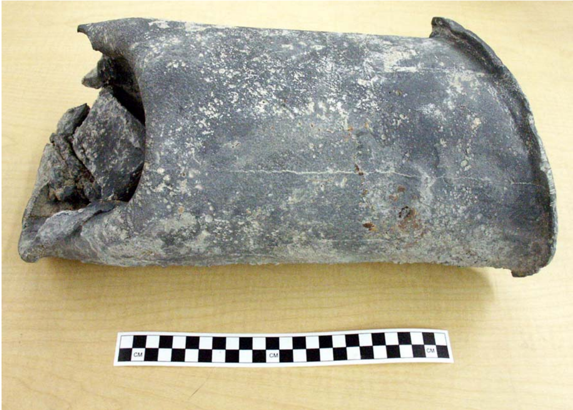
Figure 32. After face of conserved lead hawse pipe from the Mica shipwreck. Casting seams are evident on the both the external and internal surfaces (Photograph by author).
