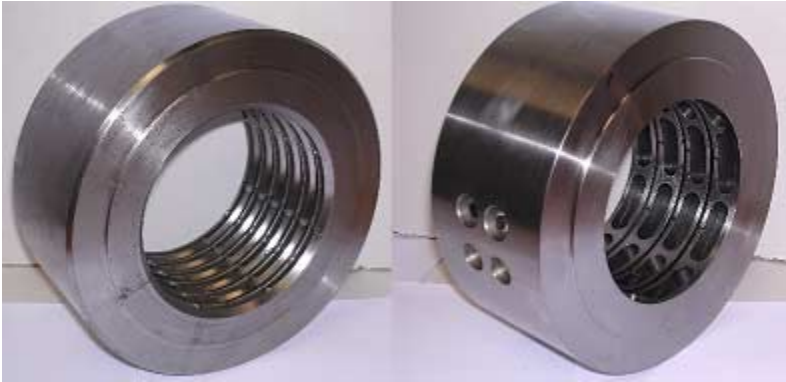
Figure 9 12-Bladed (left) and 8-Bladed (right) Pocket Damper Seals
