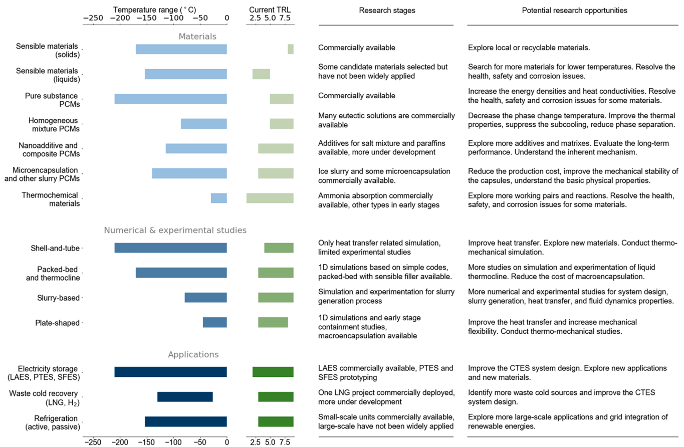
Fig. 32. Summary of temperature ranges, Technology readiness levels, research stages, and potential research opportunities of CTES studies.
