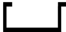
(c) Cross-section through hollow bearer in which actuation components of (a) are situated
