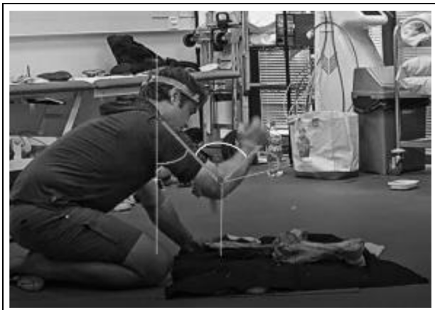
Figure 1. Photograph of experimental task. A stone tool is held in the right hand and brought into contact with a beef leg bone (the blow is aimed at the knuckle between upper and lower leg). Retroreflective markers are attached to the headband, the arm, waist and chest, for Motion Capture; wireless electromyography sensors are placed just above the elbow joint; the bone is placed on a hard, flat surface (a Kistler Force Plate covered in cloth to make cleaning easier); high-speed video cameras (positioned around the laboratory) are used to record the activity. Joint angles for biomechanical modelling are superimposed on the image.
