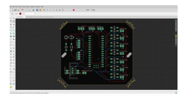
Figure 23. Eagle Circuit Board Layout
