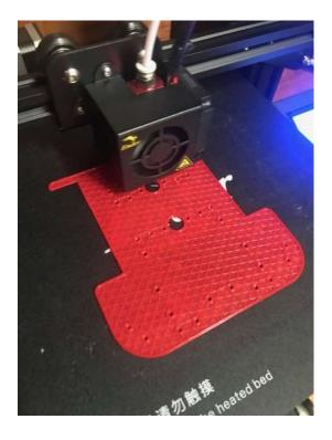
Figure 24. 3-D Printer Producing Robot Base
