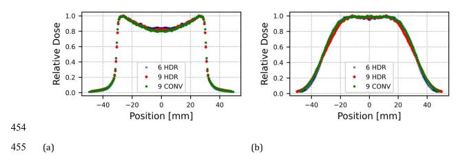
Figure S2. Profile of 6cm field at R<sub>max</sub> (a) and R30 (b) of 6 and 9 MeV UHDR, and 9 MeV CONV beams at position
