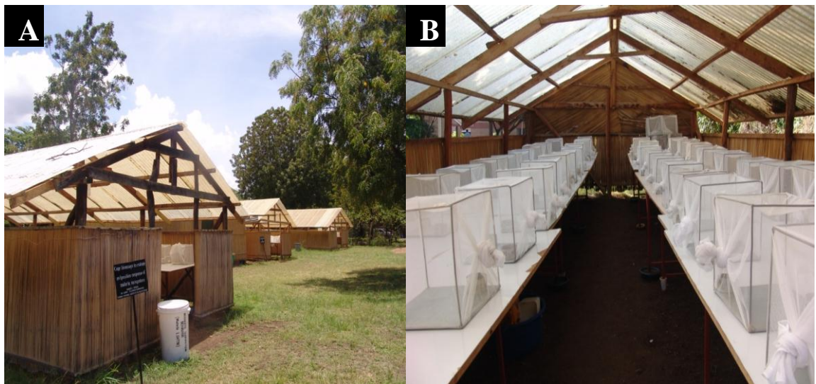
Figure 2.1. Location of egg-count bioassays. A. Sheds (10 m long \times 5 m wide \times 2.8 m high) with walls made of reed mats and a roof made of translucent corrugated polycarbonate sheets. B. Interior of a shed. In each shed two tables hold up to 25 standard cages each, allowing 40 cm of space between adjacent cages.
