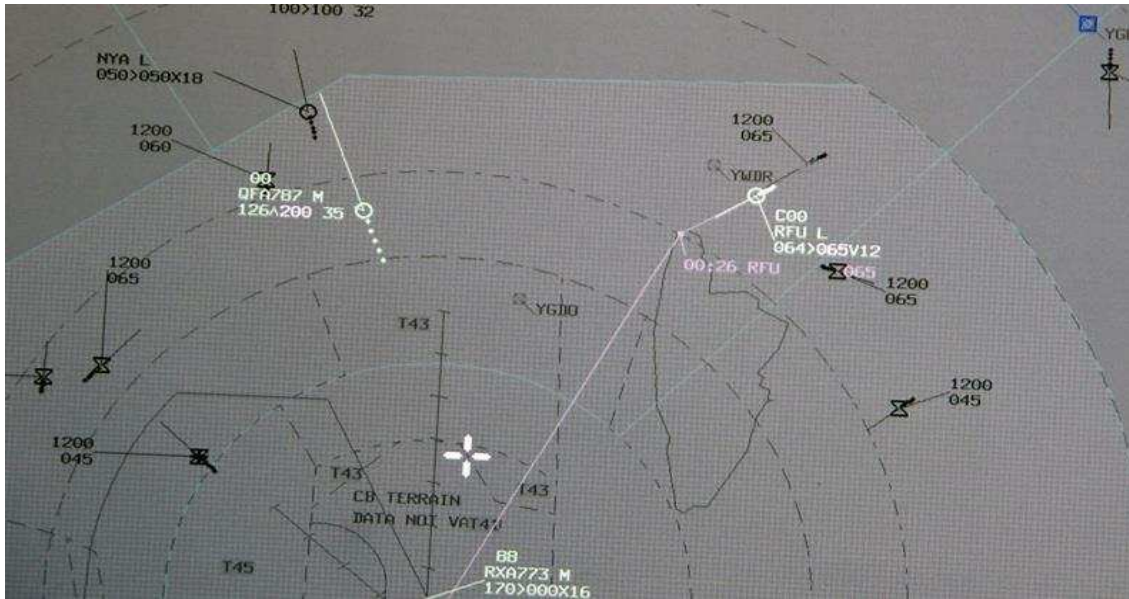
Figure 4 -1: Example of colour coded data blocks used in air traffic control, in this case from the EUROCAT air traffic control system used in the UK and many other countries (from airserviceaustralia.com , accessed 13/11/2014).
