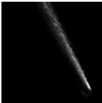
Figure 4. A single shot normalised LIF image from a fuel A spray at 250 bar. (Captured at 3.8ms after Sol)
