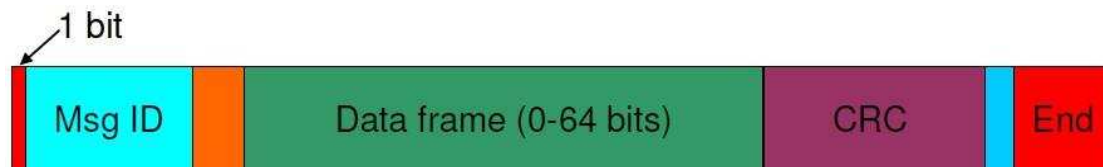
Figure 5. 8: CAN message layout [101]
