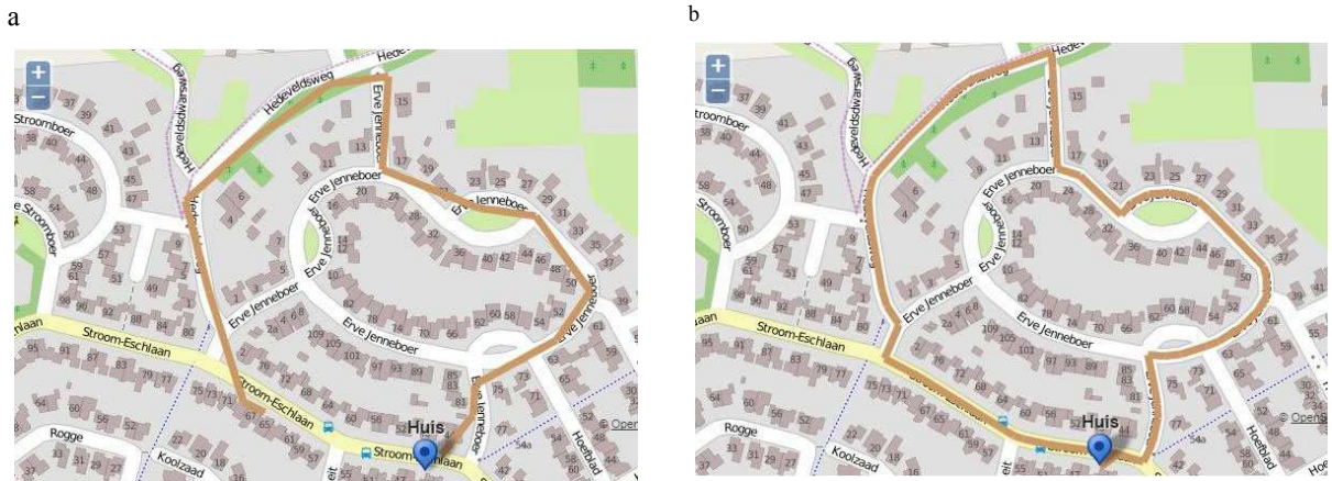
Fig. 2: (a) An example of the first stage of data processing (raw GPS data) of a measured round trip (trip length ~900 m), (b): Result of the same round trip after the second stage of processing with cleaned and map-matched data.
