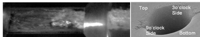
Figure 8. Left: Two counter rotating strings developed inside the nozzle hole at Full Lift, P = 4 bar, CN = 4.15 , and Re=45300 , Right: SEM image of cavitation erosion at the nozzle entrance [20].
