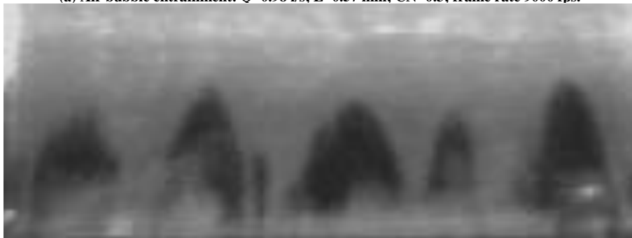
(b) Cavitation: Q=0.8 l/s; L=0.3 mm; CN=3.12 ; frame rate 18000 fps.
