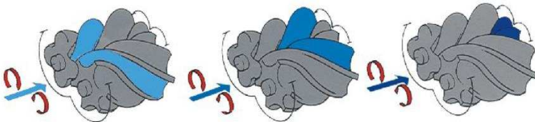
Figure 1: Screw compressor working principle
