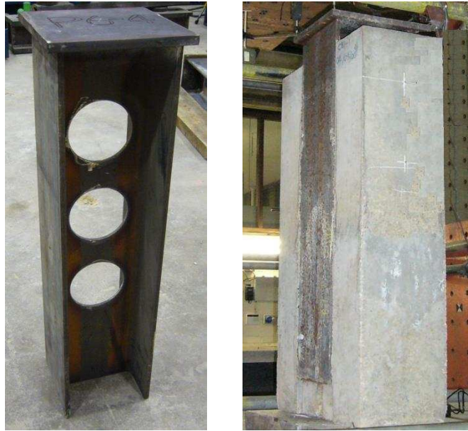
Fig. 4. Steel section and test specimen of the push-out test
