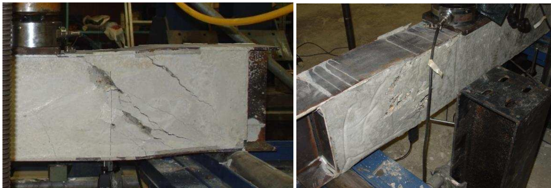
Fig. 12: USFB No.4 with concrete bursting
