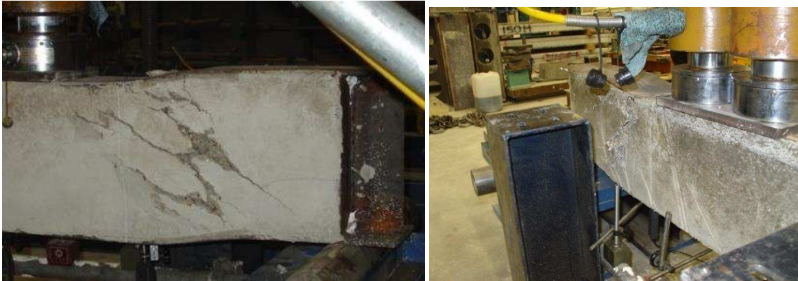
Fig. 9: USFB No.1 with concrete bursting
