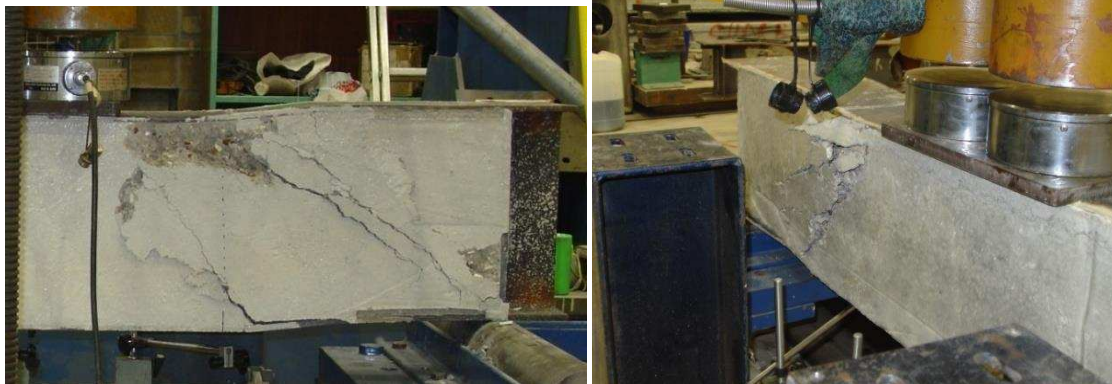
Fig. 10: USFB No.2 with concrete bursting
