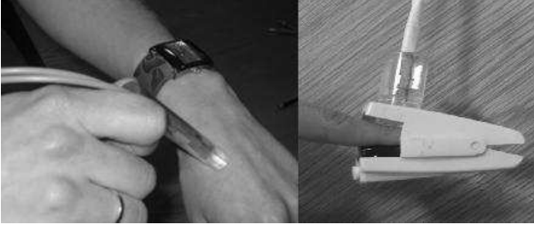
Fig. 1 (a) the developed splanchnic fibre optic probe and (b) the identical peripheral probe
