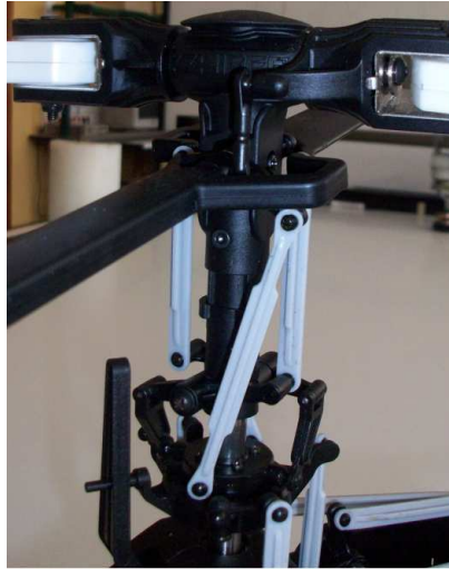
Figure 4.4: Configuration of the swashplate mechanism. Reproduced with permission from Kyosho Corporation.
