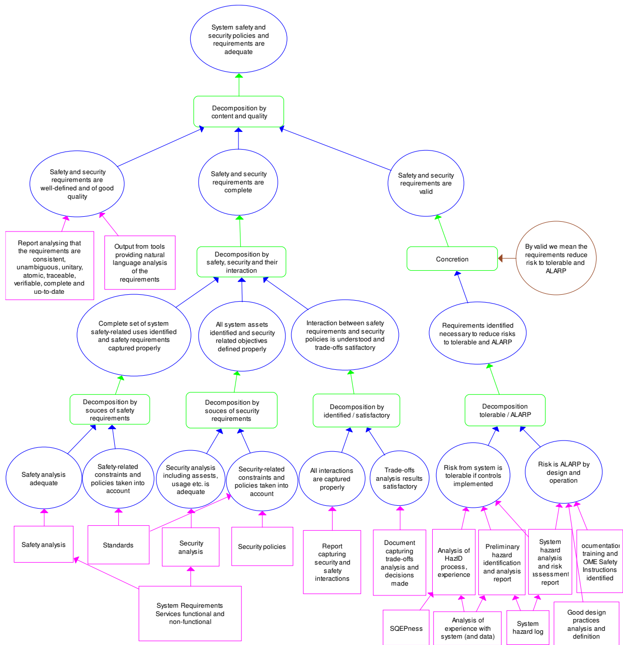
Figure 4. L0-level case fragment for the gateway in CAE notation
