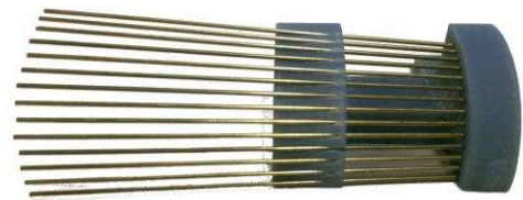
Figure 6. Guide produced by high-resolution 3D printer for precise installation of brass rods.
