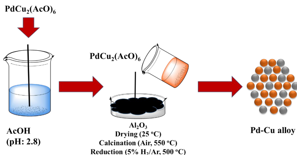
Figure 7 Representation of the preparation of \text{PdCu}_2 @ \text{Al}_2\text{O}_3 catalyst for semihydrogenation of alkynes.
