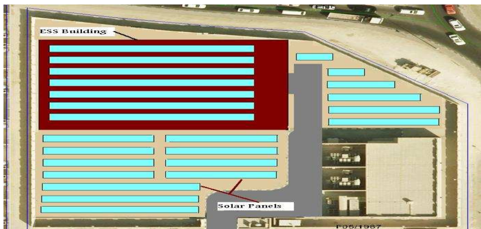
Figure 68: Conceptual layout of solar panels and BSS building in Maither North substation [7]
