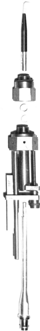
Fig. 38 DISA hot film probe : top to bottom: 55A82 probe, lower 14 mm adaptor, P.V.C. seal and retaining collar, upper adaptor with traversing screw and clamping device, and DISA probe support and cable connector.
