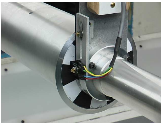
(a) Opto-coupler and input segments
