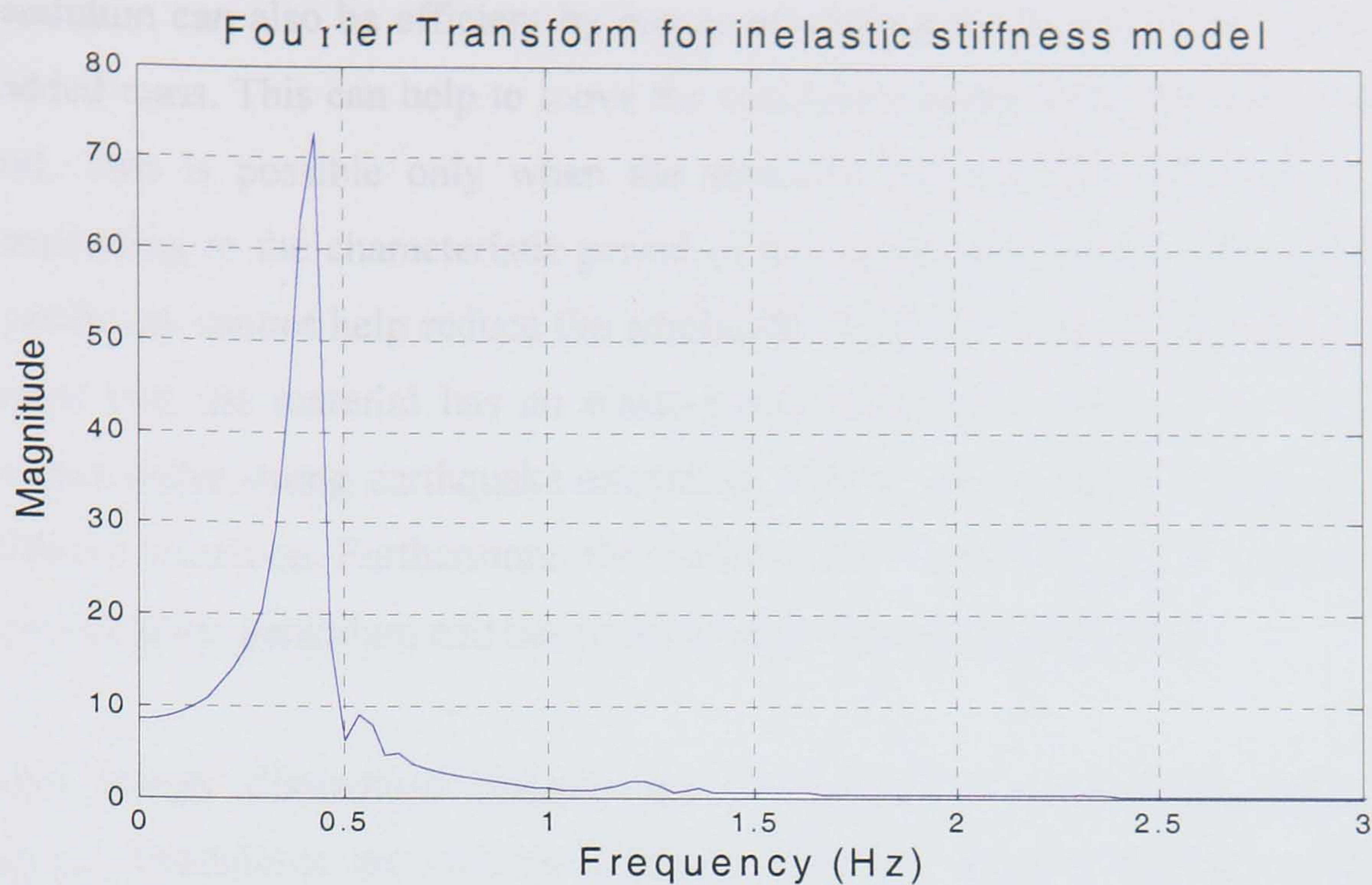
Figure 4.21 Power spectrum of inelastic stiffness model
