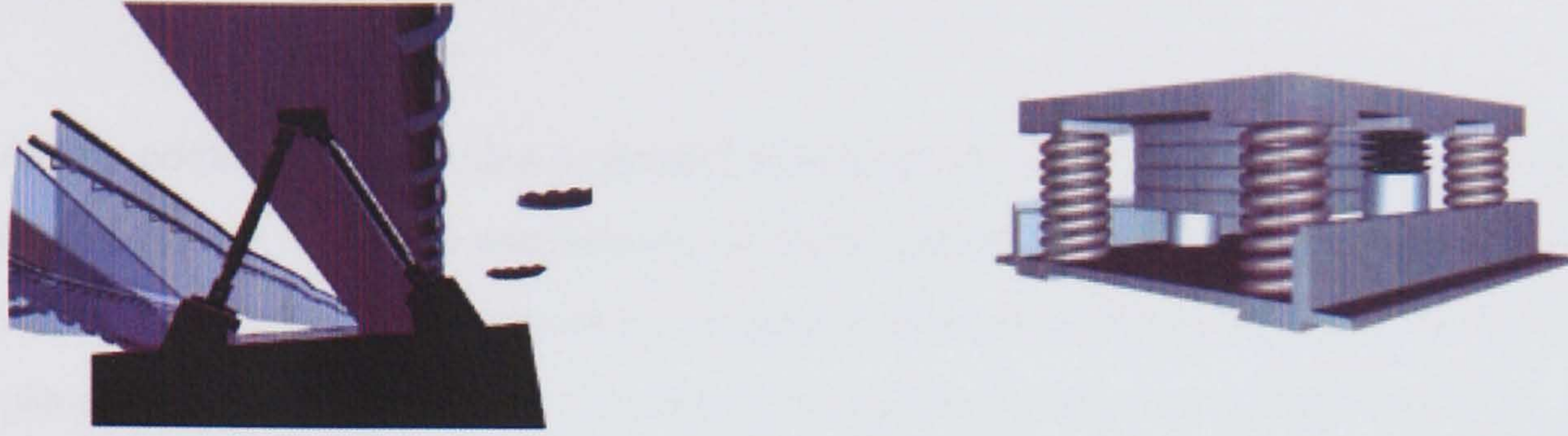
Figure 2.9. Dampers on millennium bridge Source: [Arup n.d.]
