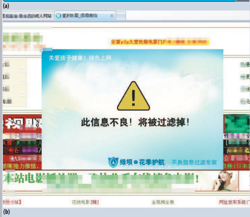
Figure 1. Green Dam Web filter. (a) Users or network administrators can choose to block or admit access to five categories of Web content. Source: University of Michigan. (b) Green Dam’s image scanner relies on skin color and face recognition to block access to pornographic websites.
