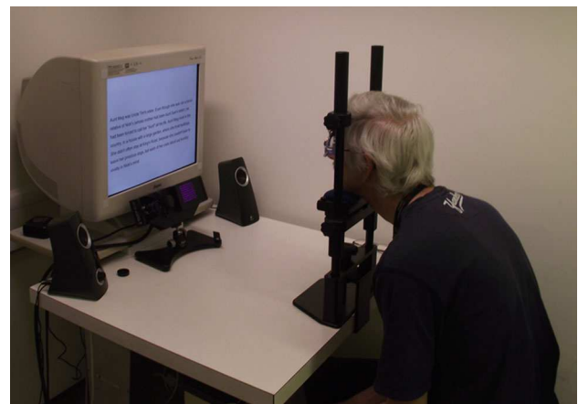
Fig. 2 The computer setup used during the reading experiment. The EyeLink 1000 eyetracking system was calibrated using the proprietary algorithm. A specified calibration accuracy of at least a “good” level (defined by the EyeLink software) was a prerequisite before each trial. Drift corrections were performed throughout experimental testing and, in cases where a large drift was detected, the subject was recalibrated before the study continued
