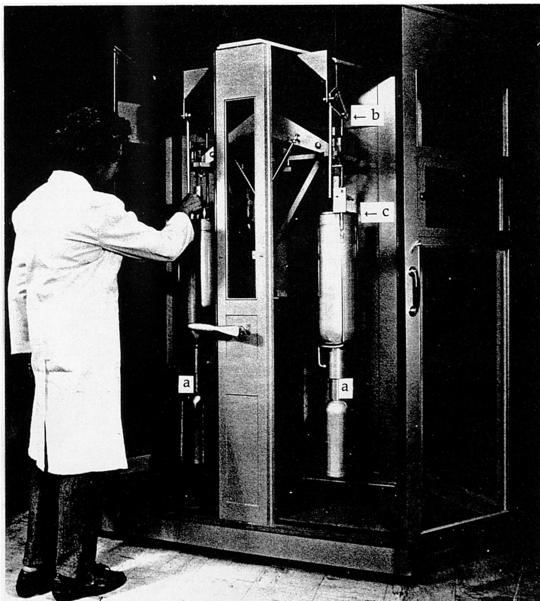
Figure 9 A photograph of the equal-arm balance used to determine the mass of collected gas, showing (a) large gas collection vessels, (b) suspension yokes, and (c) flat tops for accommodating weights (Forton and Pragnell 1985)
