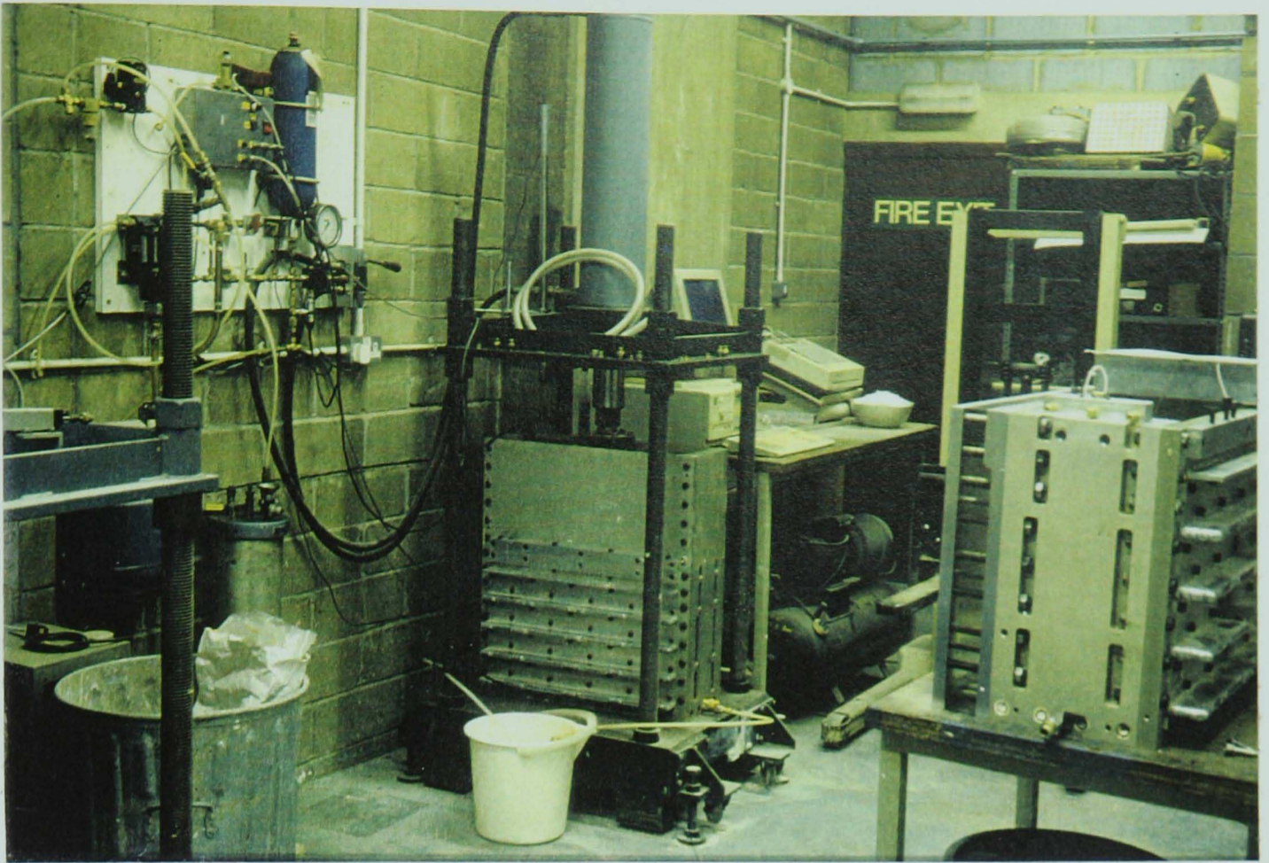
Figure 3.16 Preconsolidation of kaolin clay inside centrifuge strong-box and extension with computer controlled consolidation press
