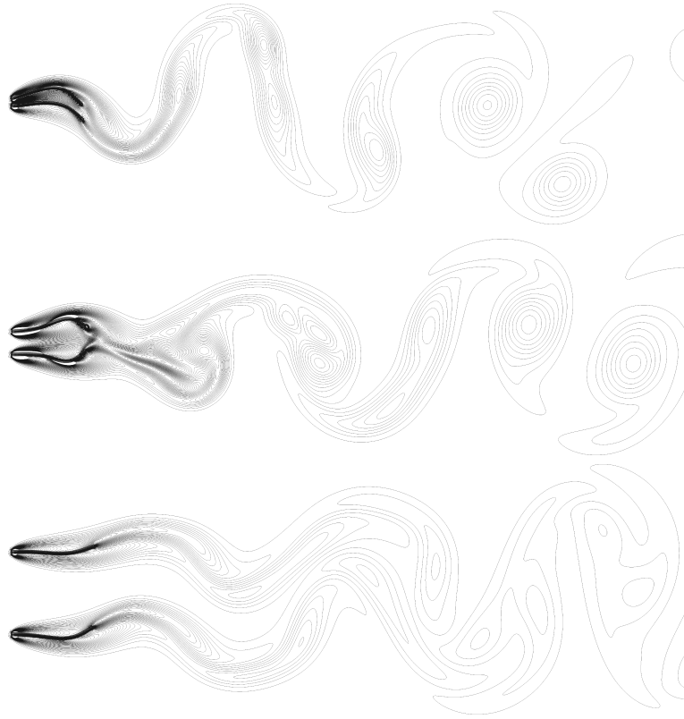
Figure 3: Snapshots of iso-vorticity for the case of two beating filaments at Re = 300 and three different spacings. (a) mode M1 at d/L = 0.1 , (b) mode M2 at d/L = 0.3 , (c) mode M2 at d/L = 1.0 .
