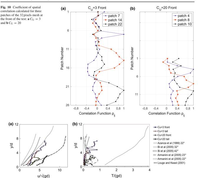
Fig. 11 Relationship between a normalised flow height against normalised velocity; b normalised flow height against granular temperature
