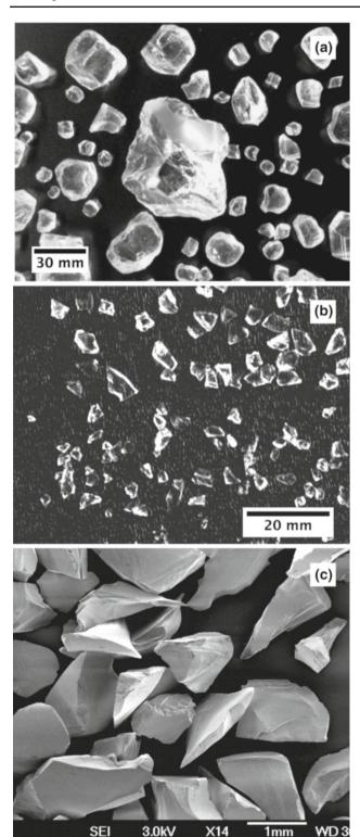
Fig. 2 Glass particles used as transparent solid. a Coarse grains; b particles finer than 4 mm; c SEM image of 600 μm particles
