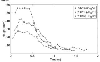
Fig. 6 Time evolution of flow heights (note truncation of flow height for PSD16 tests owing to flow thickness being larger than the image height). Circles indicate positions of meshes used for subsequent analy-
