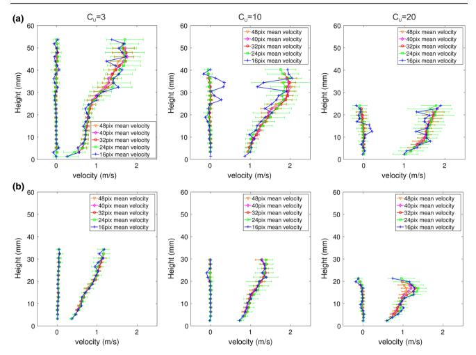
**Fig. 7** Mean velocity estimated with each patch size. **a** Results for the meshes located towards the front; **b** results for the meshes located toward the tail of the flow.  $v_x$  is on the *right* and  $v_y$  is on the *left* in each
