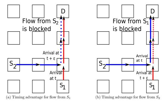
Figure 1: Small packet arrival timing offsets can determine which flow receives arbitration at contention points, potentially influencing flow latency, particularly in non-preemptive NoCs (based upon [17])
