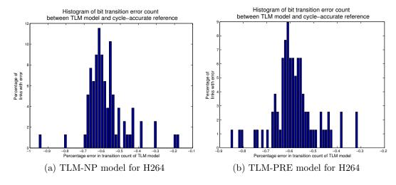
Figure 9: Histogram of link bit transition estimation errors for the TLM models relative to cycle-accurate reference for H264 application
