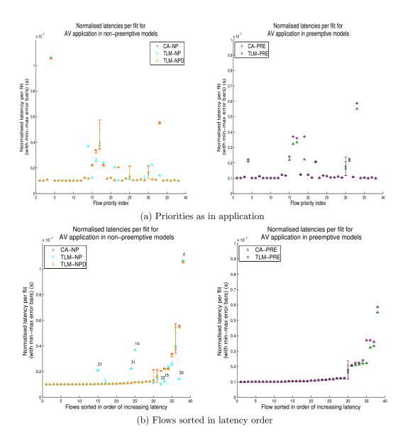
Figure 5: Latency results for the AV application under both preemptive and non-preemptive models
