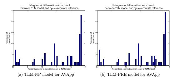
Figure 8: Histogram of link bit transition estimation errors for TLM models relative to cycle-accurate reference in AV application
