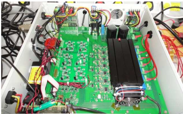
Fig. 16: Inverter with HF detection board
