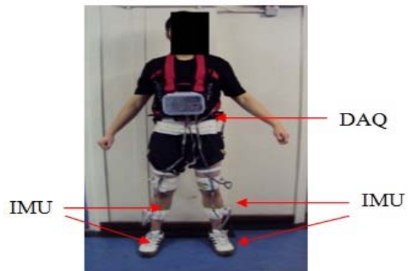
Figure-1. Setup of Gait Monitoring System.
