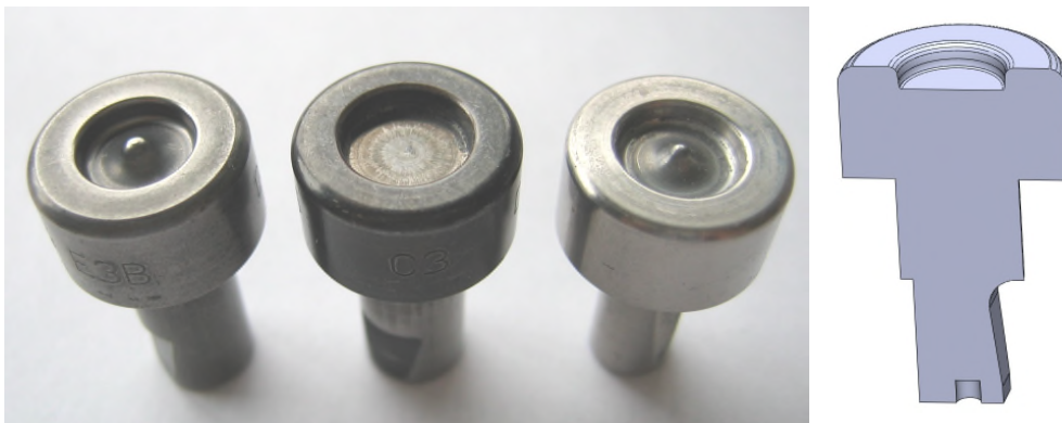
FIGURE 6. —Typical dies for SPR and a cross-section.
