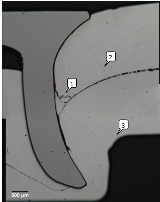
FIGURE 33. —The three crack initiation locations for a 2 mm AA5754+2 mm AA5754 stack during a T-peel fatigue [106].
