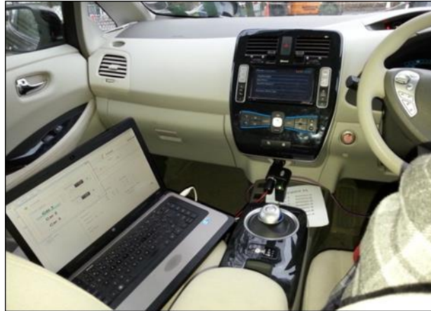
Figure 3.9 The sound delivery setup inside the target EV in the real-world experiment.
