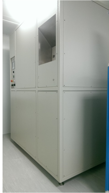
Figure 6.2: High temperature oxidation furnace in the clean room.
