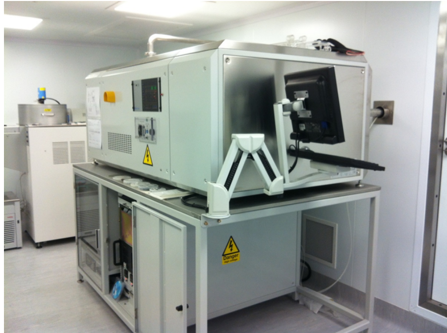
Figure 5.13: LPCVD system (Thermco Systems™) used to deposit SiO 2 on SiC.
