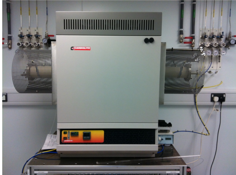
Figure 5.1: Carbolite CTF 18/300 high temperature advanced tube furnace.
