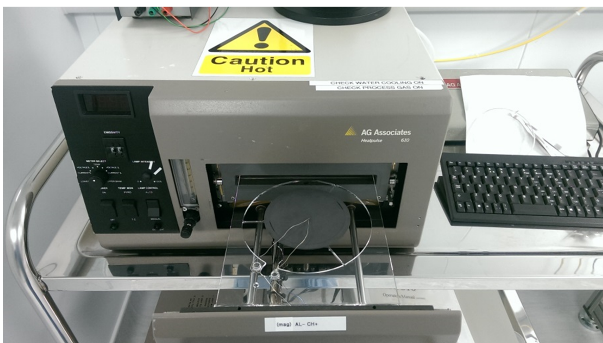
Figure 5.16: Rapid Thermal Annealing (RTA) furnace in the clean room.
