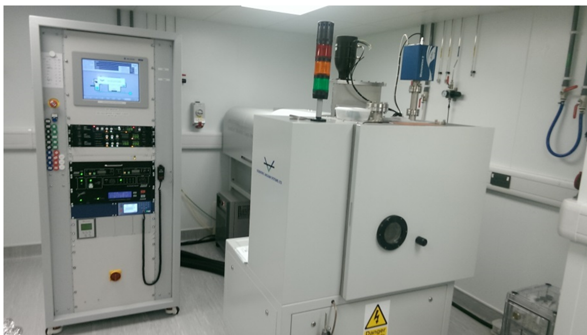
Figure 5.15: Electron Beam Evaporator Deposition system.
