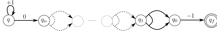
■ Figure 1 Illustration of the BVASS_1 \mathcal{B}_n . The reachability set of the control state q_n is the singleton set \{2^n\} , and a reachability tree for q(0) contains all counter values between 0 and 2^n .
