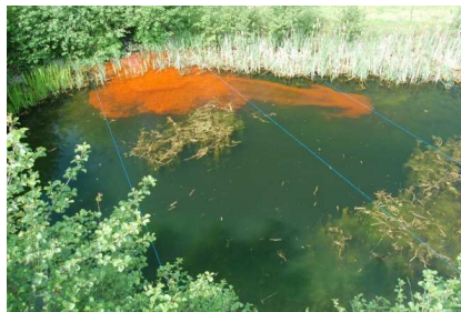
Fig. 1 Tracer study used for flow visualization in a treatment pond. Image courtesy of Hart et al. , 2014.
